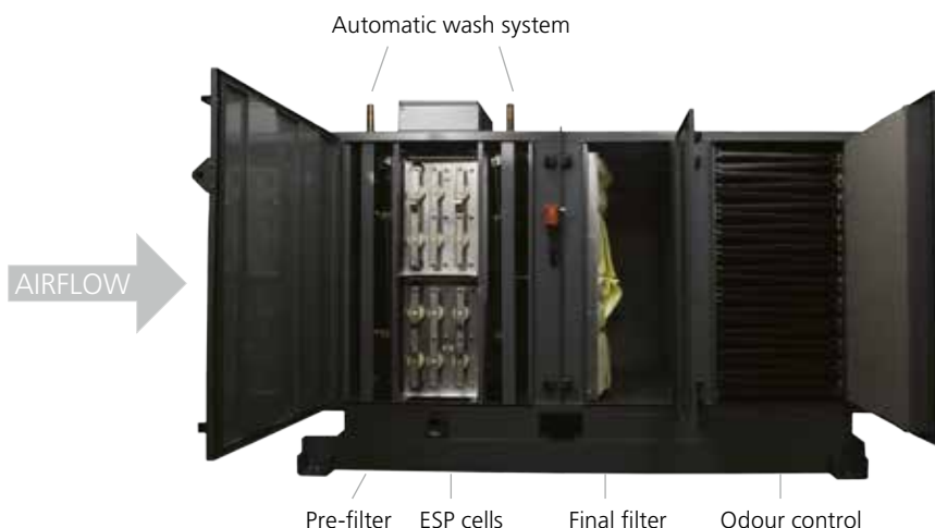
Figure 8: A typical automatic wash ESP.
